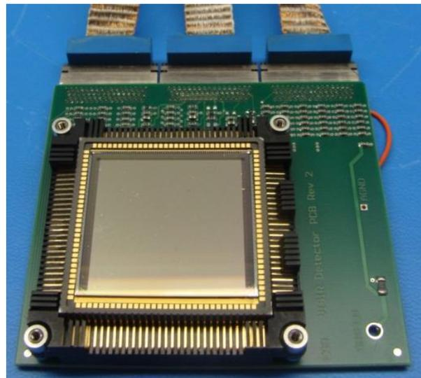
Figure 3b: AQUARIUS MUX mounted in its socket
