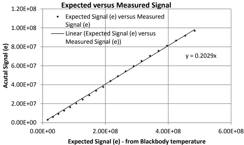
Figure 2 - System throughput measured, expected signal versus measured signal for increasing blackbody temperature.
