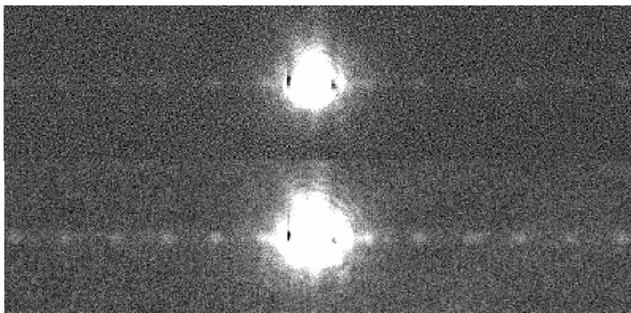
Figure 6 - Top frame is the 1 Hz frequency chopped image and the bottom frame is the 10 Hz chopped image, for a pinhole image projected onto the detector and with the use of a chopper wheel to mimic the telescope chopping.
