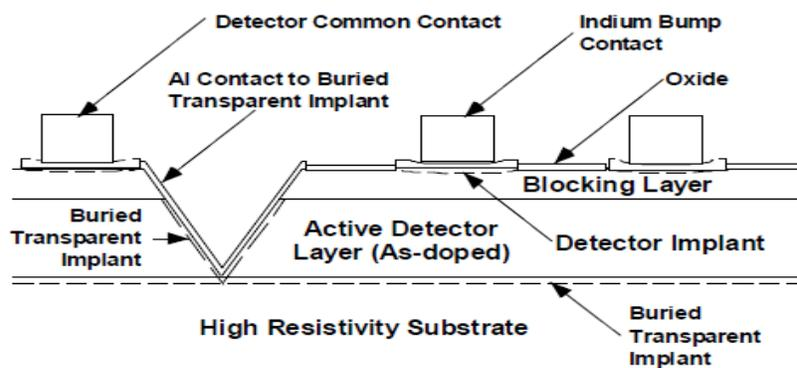
Figure 9 - Basic architecture of a back illuminated IBC detector, from the AQUARIUS detector user manual.
