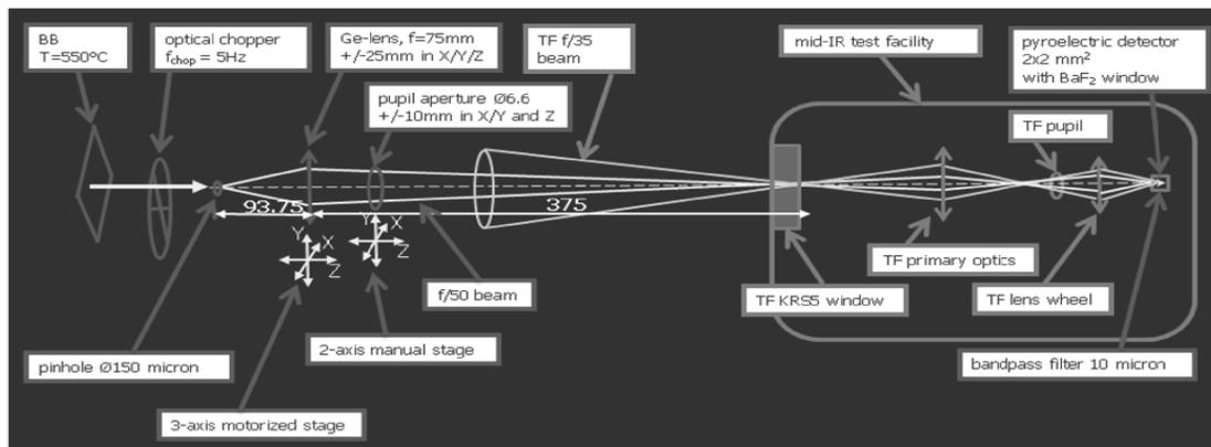
Figure 3 – Optical test setup to determine system optical throughput of test cryostat at room temperature
