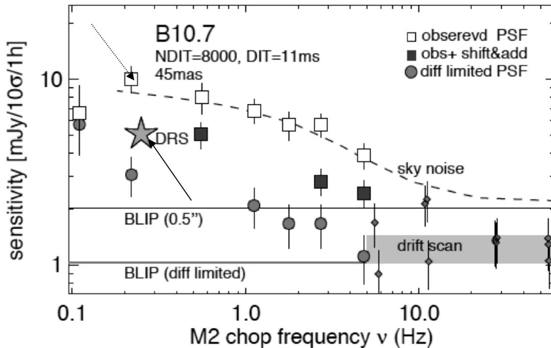
Figure 1- VISIR sensitivities as a function of telescope chop frequency. Observations obtained with B10.7 filter on standard star HD198048. Star point and straight arrow indicates sensitivity of VISIR with old DRS detector at chop frequency of 0.25Hz. White square with dotted arrow shows sensitivity with the new AQUARIUS detector versus telescope chop frequency, at 0.25Hz it is almost twice as bad. Other points not relevant to this paper.
