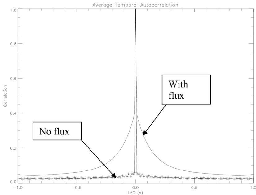
Figure 10 - **Temporal auto-correlation measurement for detector showing correlation as a function of time**, for high flux the correlation is clearly seen and for no flux (+), there is no correlation seen and thus no ELFN.
