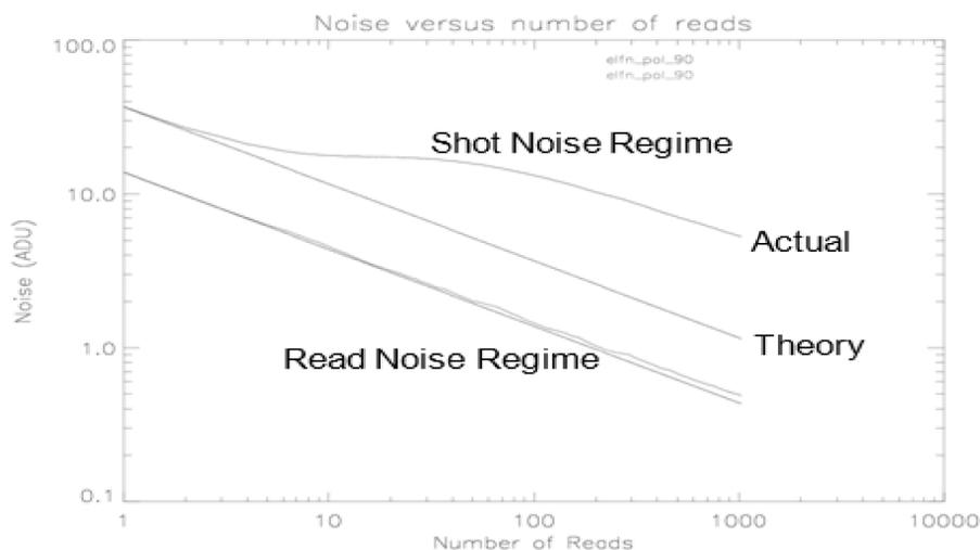
Figure 4 - plots of measured noise versus number of co-added reads for both the low flux and high flux regimes. The straight lines indicate the corresponding theoretical values.
