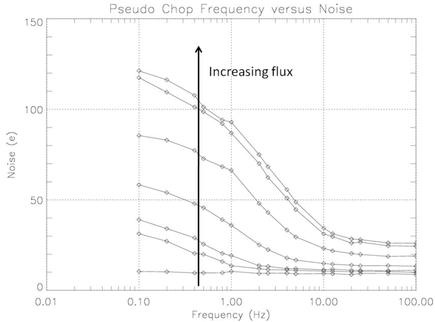
Figure 5 - Detector noise versus “pseudo” chop frequency (chop is produced in software) for increasing flux levels
