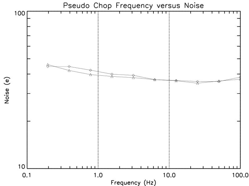
Figure 8 - Noise as a function of frequency for the AQUARIUS MUX when at operational temperature, plots given for two d.c. levels to mimic different signal levels (triangle is low signal level and diamond is high signal level).
